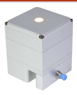
The ARCoptix ARCSPHERE is an integrating sphere featuring an internal halogen light source for diffuse reflection measurements in the VIS-NIR. The highly reflective sphere has a diameter of 50mm, a sample port of 10mm with a sapphire window, and includes an SMA fiber connector allowing a direct connection to the spectrometer. The internally illuminated design provides a much stronger signal (at least 50 times more) than spheres illuminated via fiber optic coupled light sources.
